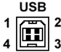
Figure 3-4: USB Connector pin orientation.
